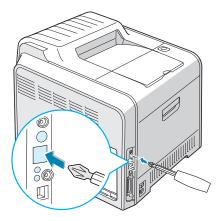
If you replace the network interface card with a new one, remove the two screws and the old card.
